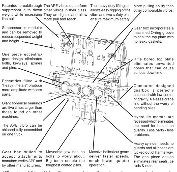
APE provides a full line of high quality power units but our vibros will run off most correct sized power units.
